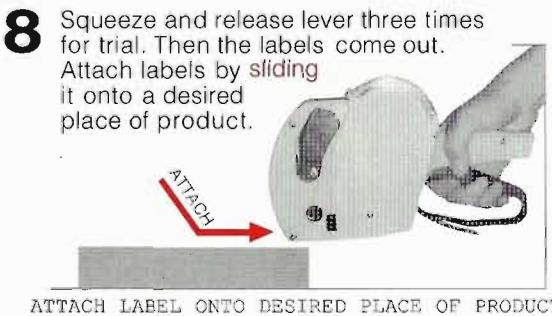
8 Squeeze and release lever three times for trial. Then the labels come out. Attach labels by sliding it onto a desired place of product.
