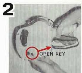
2 Pull out Base Plate by pulling back Plate Open Keys on both sides of labeler.
