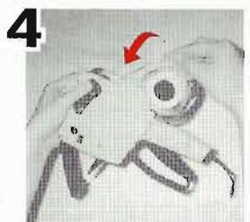
4 Insert Roll into Tunnel above "LABEL" sign until you see 10cm of label paper coming out at the bottom. Then close Label Roll Cover.
